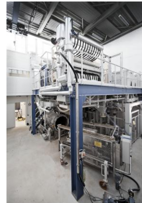
The new pilot plant produces 100 kg of Celitement ® daily. (Photo: Markus Breig)
